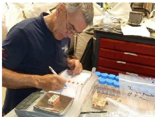
Photo 6 : Weighing of the test specimens for the later determination of their moisture content
