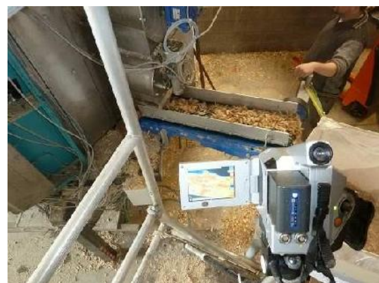
Photo 12 : System of photography using an infra-red camera
