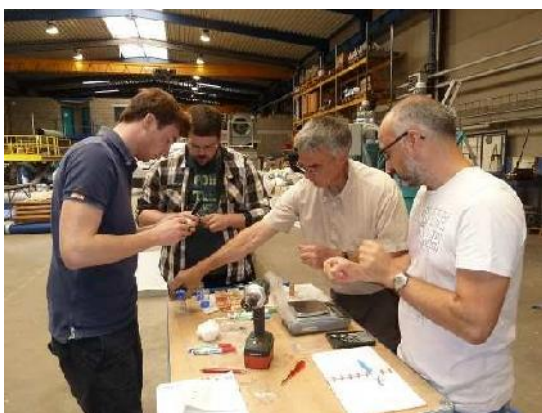
Photo 5 : Sealing of the lodgements by means of a cotton plug, marking of the test specimens
