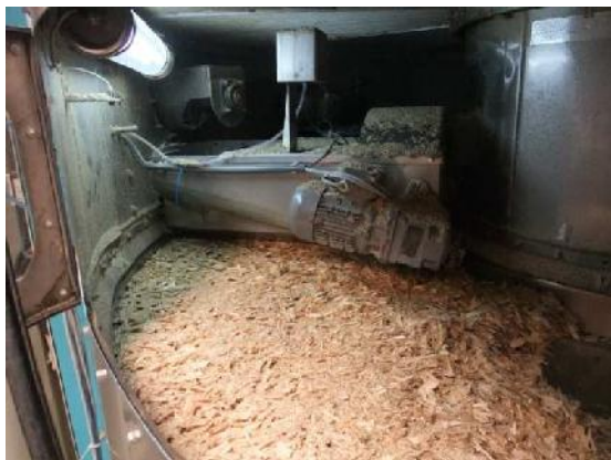
Photo 9 : Homogeneous layer of chips on the upper disc
