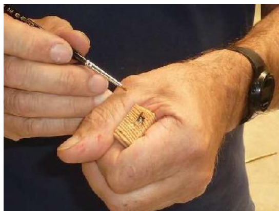
Photo 4 : Introduction of a larva into a lodging drilled into the transverse face of the test specimen
