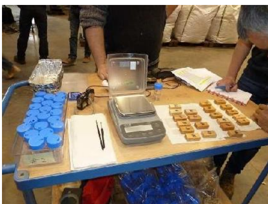
Photo 3 : Preparation of the test specimens (larvae, precision balance and test specimens)
