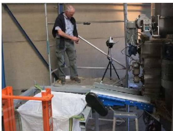
Photo 11 : Arrangement of the infra-red camera above the conveyor belt
