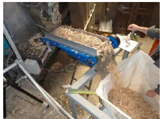
Photo10 : Evacuation of the chips at the output of the oven on a conveyor belt
