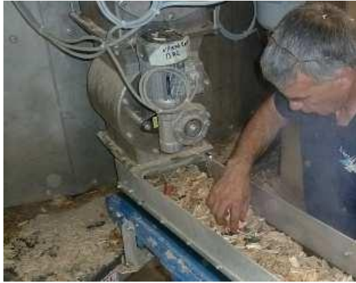
Photo 13 : Recovery of the test specimens mixed with the chips
